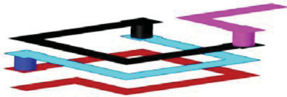
Fig. 1. Typical helical inductor made from thin metal traces.
