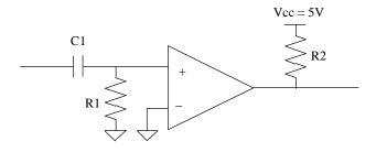
Assume the comparator is an LM2903<sup>1</sup>, for which the output is an open-collector type and the input bias current is 25 nA. Values are needed for the resistors and capacitor.
